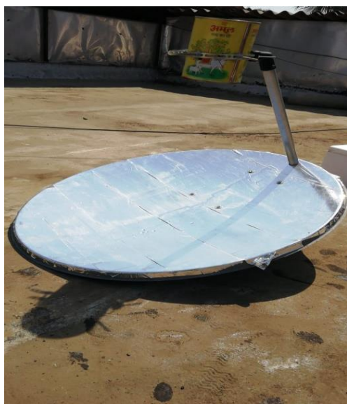
Fig. 3. Parabolic type solar concentrator
